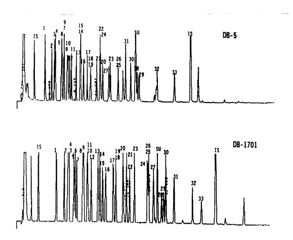
GC/ECD chromatogram of the PFB derivatives of phenolic compounds analyzed on a DB-5/DB-1701 fused-silica open-tubular column pair. The GC operating conditions were as follows: 30 m x 0.53 mm ID DB-5 (0.83  $\mu$ m film thickness) and 30 m x 0.53 mm ID DB-1701 (1.0  $\mu$ m film thickness) connected to an 8" injection tee (Supelco Inc.). Temperature program: 150°C (1 min hold) to 275°C (2 min hold) at 30°C/min.
