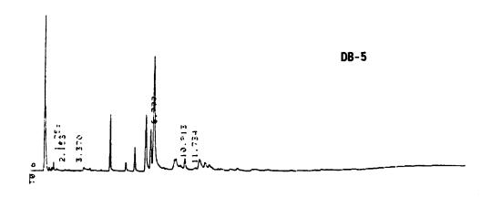
FIGURE 2. GC/ECD chromatogram of Aroclor 1221 analyzed on a DB-5/DB-1701 fused-silica open-tubular column pair. The GC operating conditions were as follows: 30 m x 0.53 mm ID DB-5 (1.5-µm film thickness) and 30 m x 0.53 mm ID DB-1701 (1.0-µm film thickness) connected to a J&W Scientific press-fit Y-shaped inlet splitter. Temperature program: 150°C (0.5 min hold) to 190°C (2 min hold) at 12°C/min then to 275°C (10 min hold) at 4°C/min.
