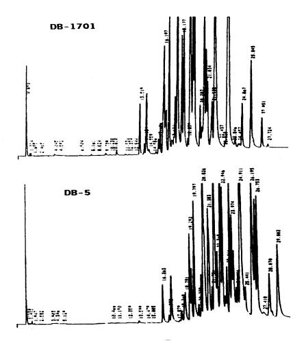
FIGURE 7. GC/ECD chromatogram of Aroclor 1260 analyzed on a DB-5/DB-1701 fused-silica open-tubular column pair. The GC operating conditions were as follows: 30 m x 0.53 mm ID DB-5 (1.5-µm film thickness) and 30 m x 0.53 mm ID DB-1701 (1.0-µm film thickness) connected to a J&W Scientific press-fit Y-shaped inlet splitter. Temperature program: 150°C (0.5 min hold) to 190°C (2 min hold) at 12°C/min then to 275°C (10 min hold) at 4°C/min.
