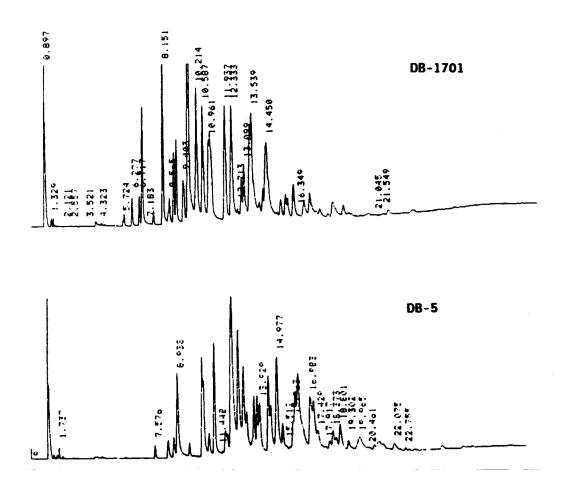
FIGURE 4. GC/ECD chromatogram of Aroclor 1242 analyzed on a DB-5/DB-1701 fused-silica open-tubular column pair. The GC operating conditions were as follows: 30 m x 0.53 mm ID DB-5 (1.5-µm film thickness) and 30 m x 0.53 mm ID DB-1701 (1.0-µm film thickness) connected to a J&W Scientific press-fit Y-shaped inlet splitter. Temperature program: 150°C (0.5 min hold) to 190°C (2 min hold) at 12°C/min then to 275°C (10 min hold) at 4°C/min.
