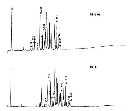
FIGURE 1. GC/ECD chromatogram of Aroclor 1016 analyzed on a DB-5/DB-1701 fused-silica open-tubular column pair. The GC operating conditions were as follows: 30 m x 0.53 mm ID DB-5 (1.5-µm film thickness) and 30 m x 0.53 mm ID DB-1701 (1.0-µm film thickness) connected to a J&W Scientific press-fit Y-shaped inlet splitter. Temperature program: 150°C (0.5 min hold) to 190°C (2 min hold) at 12°C/min then to 275°C (10 min hold) at 4°C/min.
