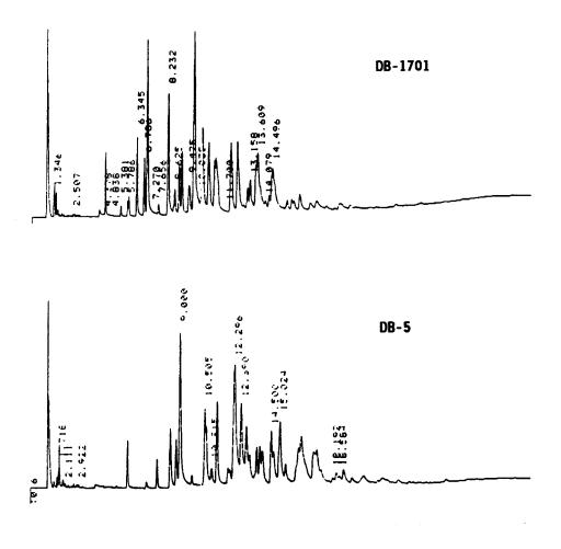
FIGURE 3. GC/ECD chromatogram of Aroclor 1232 analyzed on a DB-5/DB-1701 fused-silica open-tubular column pair. The GC operating conditions were as follows: 30 m x 0.53 mm ID DB-5 (1.5-µm film thickness) and 30 m x 0.53 mm ID DB-1701 (1.0-µm film thickness) connected to a J&W Scientific press-fit Y-shaped inlet splitter. Temperature program: 150°C (0.5 min hold) to 190°C (2 min hold) at 12°C/min then to 275°C (10 min hold) at 4°C/min.
