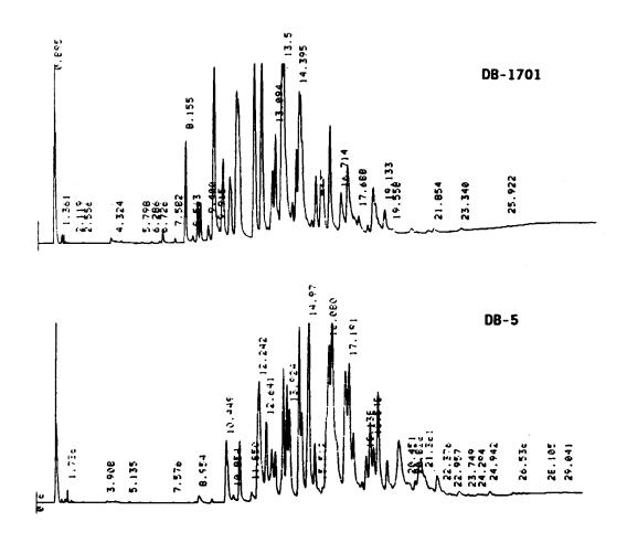
FIGURE 5. GC/ECD chromatogram of Aroclor 1248 analyzed on a DB-5/DB-1701 fused-silica open-tubular column pair. The GC operating conditions were as follows: 30 m x 0.53 mm ID DB-5 (1.5-µm film thickness) and 30 m x 0.53 mm ID DB-1701 (1.0-µm film thickness) connected to a J&W Scientific press-fit Y-shaped inlet splitter. Temperature program: 150°C (0.5 min hold) to 190°C (2 min hold) at 12°C/min then to 275°C (10 min hold) at 4°C/min.
