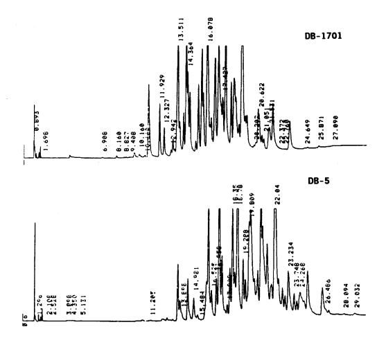
FIGURE 6. GC/ECD chromatogram of Aroclor 1254 analyzed on a DB-5/DB-1701 fused-silica open-tubular column pair. The GC operating conditions were as follows: 30 m x 0.53 mm ID DB-5 (1.5-µm film thickness) and 30 m x 0.53 mm ID DB-1701 (1.0-µm film thickness) connected to a J&W Scientific press-fit Y-shaped inlet splitter. Temperature program: 150°C (0.5 min hold) to 190°C (2 min hold) at 12°C/min then to 275°C (10 min hold) at 4°C/min.
