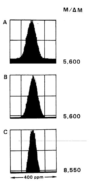
Peak profile displays demonstrating the effect of the detector zero on the measured resolving power. In this example, the true resolving power is 5,600.
