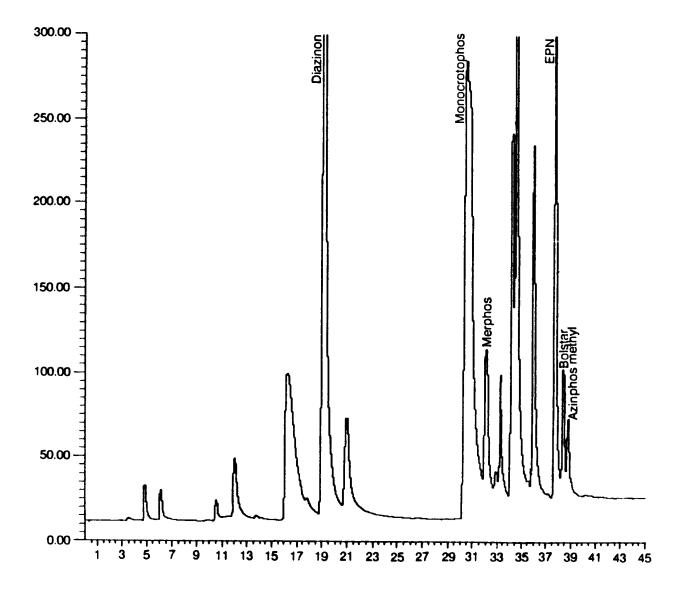
Figure 4. Chromatogram of target organophosphorus compounds from a 15-m DB-210 column with NPD detector. More compounds are shown in Figure 3. See Table 3 for retention times.
