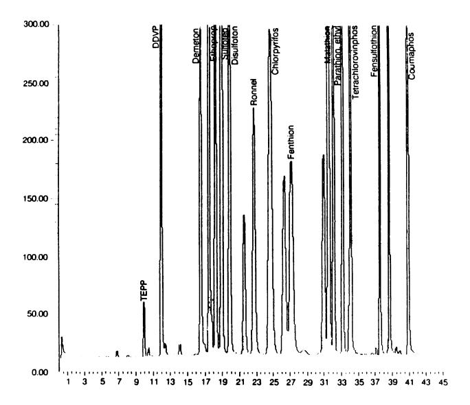
Figure 1. Chromatogram of target organophosphorus compounds from a 15-m DB-210 column with FPD detector. More compounds are shown in Figure 2. See Table 3 for retention times.
