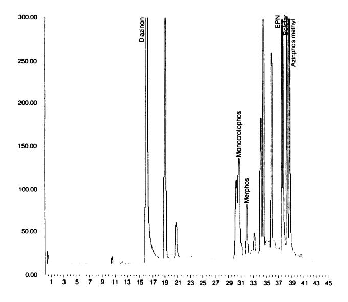
Figure 2. Chromatogram of target organophosphorus compounds from a 15-m DB-210 column with FPD detector. More compounds are shown in Figure 1. See Table 3 for retention times.
