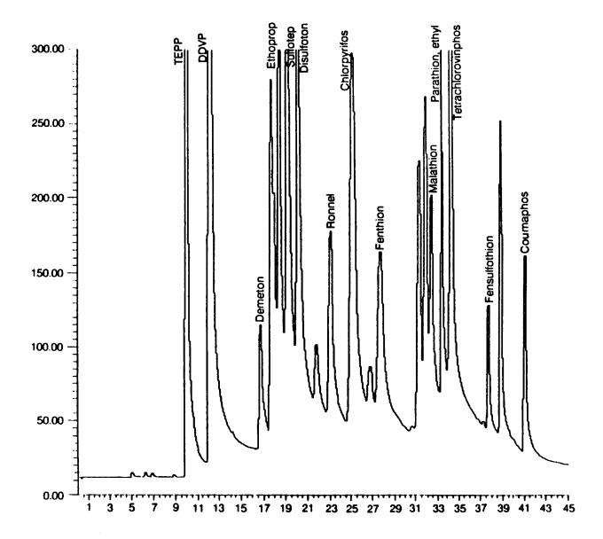
Figure 3. Chromatogram of target organophosphorus compounds from a 15-m DB-210 column with NPD detector. More compounds are shown in Figure 4. See Table 3 for retention times.
