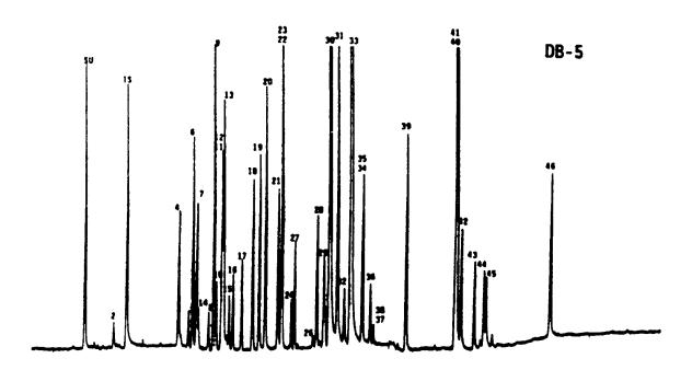
Figure 5. Chromatogram of target organophosphorus compounds on a 30-m DB-5/DB-210 column pair with NPD detector, without Simazine, Atrazine and Carbophenothion. See Table 4 for retention times and for GC operating conditions.
