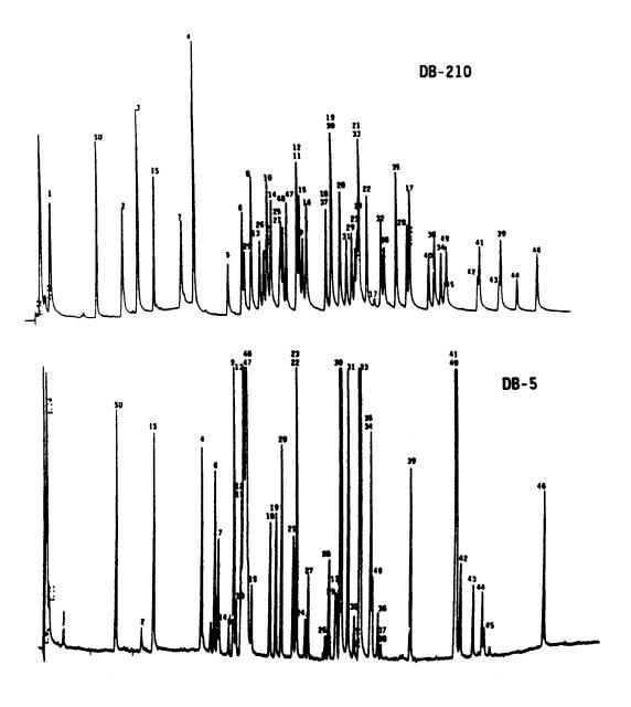
Figure 6. Chromatogram of target organophosphorus compounds on a 30-m DB-5/DB-210 column pair with NPD detector, with Simazine, Atrazine and Carbophenothion. See Table 4 for retention times and for GC operating conditions.
