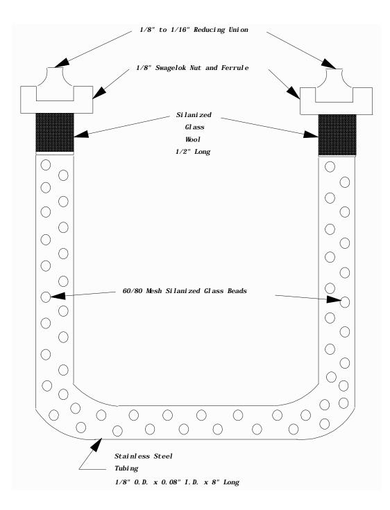
FIGURE 5. CRYOGENIC TRAP DESIGN
